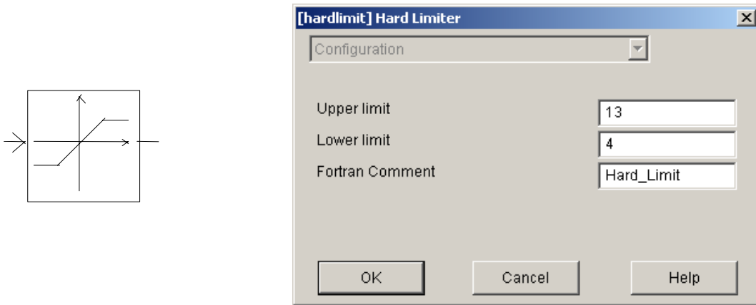
Figure 52: Hard limiter characteristics
